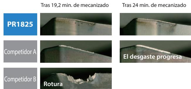
Condiciones de corte :  $V_c = 150$  m/min,  $a_p \times a_e = 2$  mm x 65 mm,  $f_z = 0.12$  mm/t, SKD11, Sin refer. PNMU1205ANER-GM (MFPN45)
