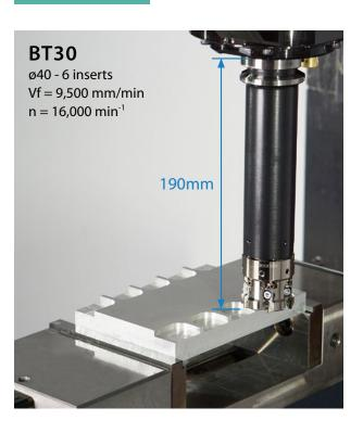
$n = 16,000 \text{ min}^{-1} (Vc = 2,000 \text{ m/min})$  Vf = 9,500 mm/min (fz = 0.1 mm/t) ap x ae = 5 x 5 mm ADC12 Wet ø40 (6 inserts) MD90-040RS-T6CMSF LNGX180704PDFR-RR (KPD01A) (Internal evaluation)
