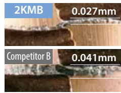
Cutting edge condition (After 62 minutes machining)
